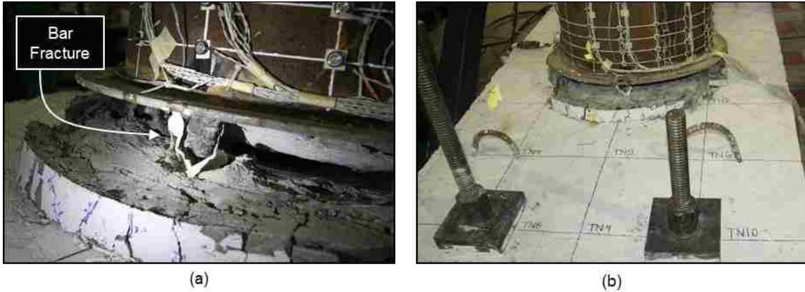
Figure 5.48: WRCUB (a) North bar fracture, and (b) North cap beam damage at 12.27% drift South
