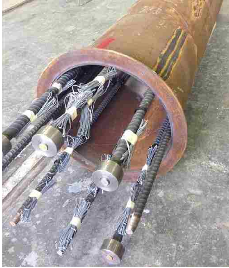
Figure 4.11: Specimen WRC annular ring and reinforcing bars
