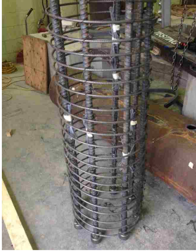
Figure 4.13: Reinforcing cage of Specimen RC
